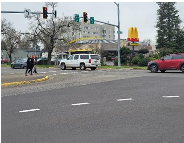
Fig. 2 At No-All-Red, the red SUV is clearing the intersection during the first second of the red clearance interval while two pedestrians are crossing during the “Walk” interval concurrently.
