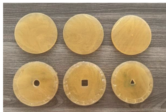
Fig. 1 At the top, undamaged Araldite plates; at the bottom, damaged plates with triangular, square, and circular geometries.
