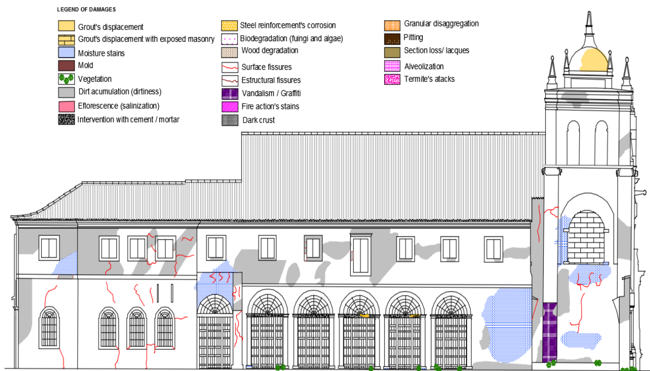
Fig.11 Damage's Map of Our Lady of Carmo's Church – East Facade..
