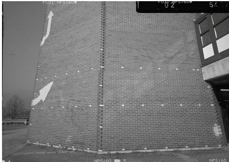
Fig. 1 UAV image of test field—high-resolution UAV image of two intersecting brick walls with red-brown bricks and white mortar, used for photogrammetric.
