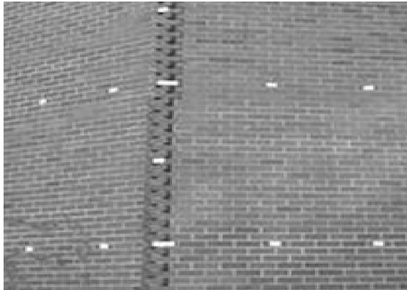
Fig. 2 Check point distribution—Distribution of 100 brick-corner check points across the test field for accuracy assessment.
