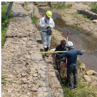
Fig. 5 Deformation measurement at site.
