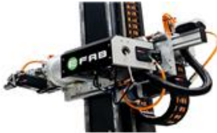
Figure 10. Robot carpet tufting tool.
