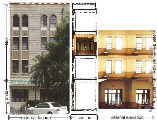
Fig. 1 Diagram of the claddings of the partly southern elevation, the section with horizontal circulations and the opposite internal elevation of the TPH.
