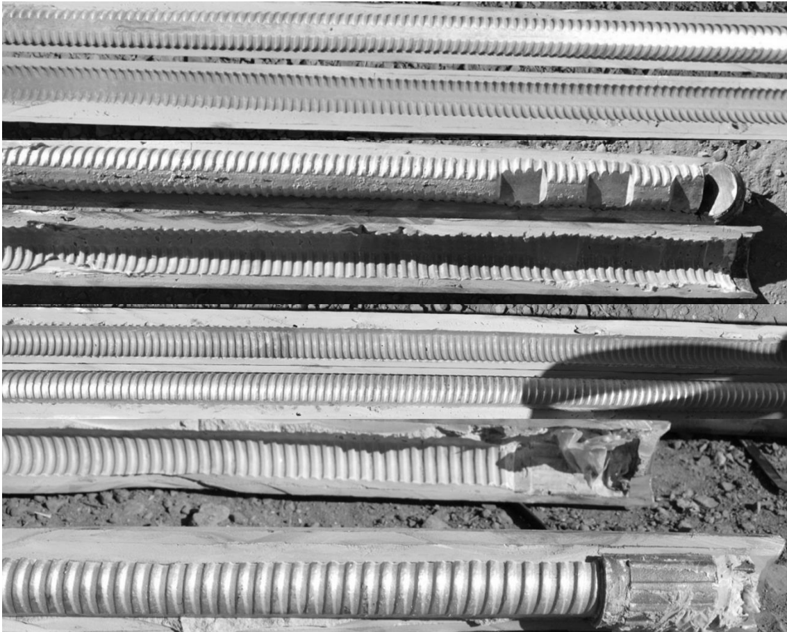
Fig. 11 Resin mixing results from testing completed. (a) One example of the resin mixing completed using the paddle mixing device; (b) One example of the resin mixing completed using the resin shredder mixing.
