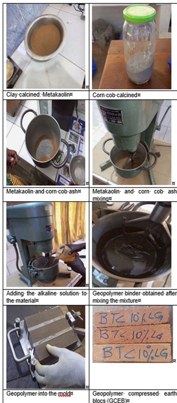
Fig. 1 Principle for geopolymer synthesis.
