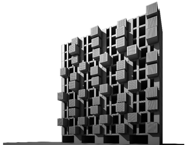
Fig. 10 High-rise precast concrete social housing.
