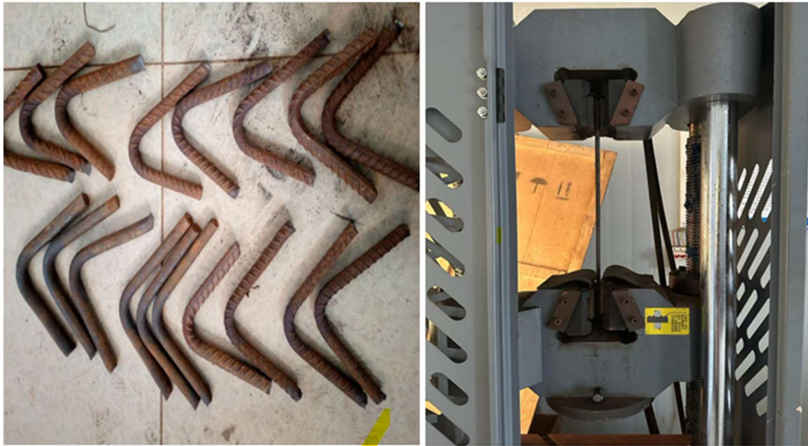
Fig. 4 The iron bars after bending and the apparatus used for tensile and bending tests.
