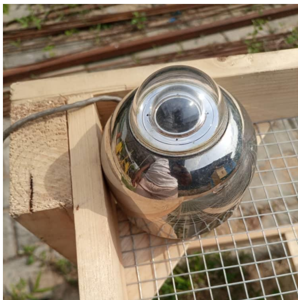
Fig. 6 The EPPLEY type pyranometer.
