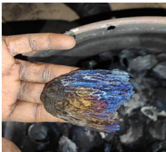
Fig. 20 Charcoal obtained after the first experiment.
