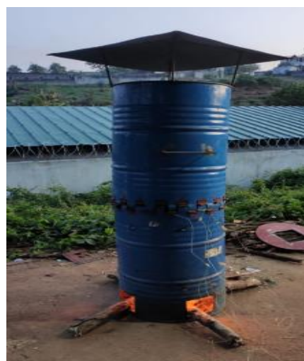
Fig. 9 The carbonization stove used for the pyrolysis of the shells.
