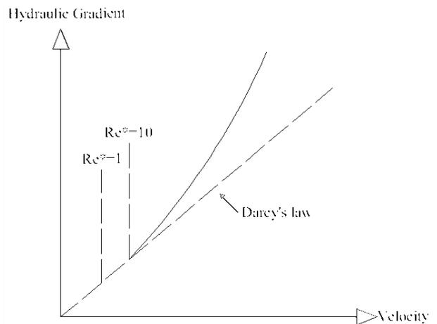
**Fig. 2** Schematic curve relating hydraulic gradient and velocity.
