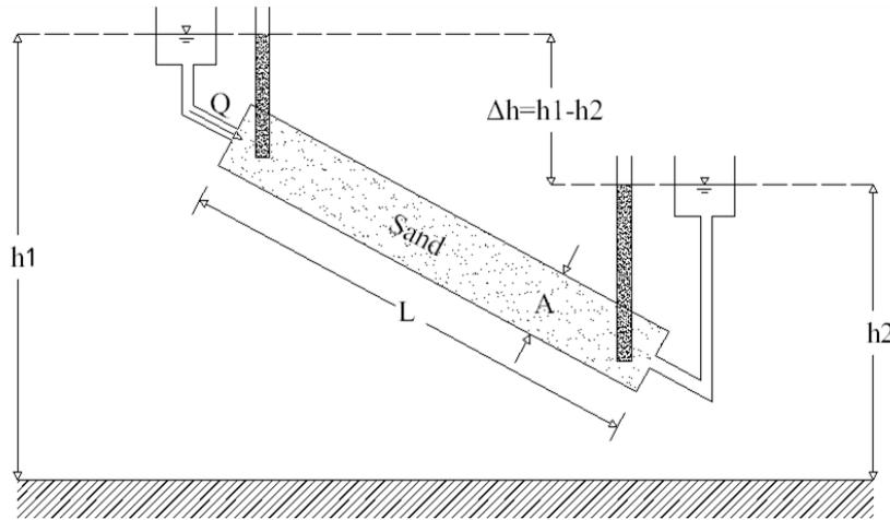
**Fig. 1** Darcy's apparatus.
