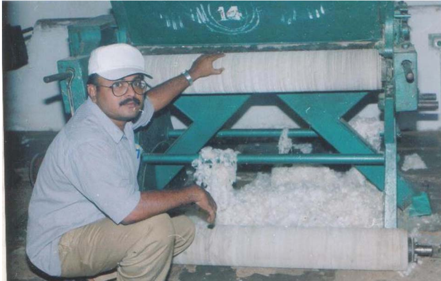
ECO-FRIENDLY ROLLER GIN OF DESIGN-V , WHICH FAILED TO OPERATE SUCCESSFULLY GINNING SEED- COTTON
