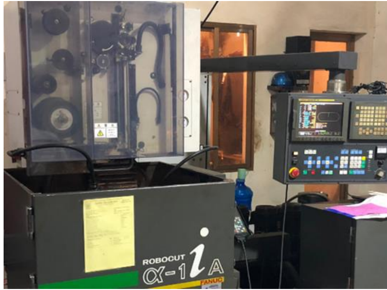
Fig. 2 Wire-EDM machine used in the experiment.
