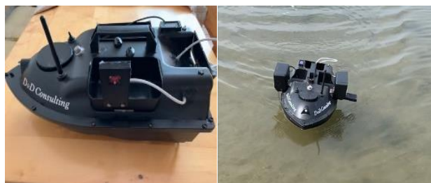
Fig. 5 Radio controlled water drone equipped with probe and a spectrophotometer.
