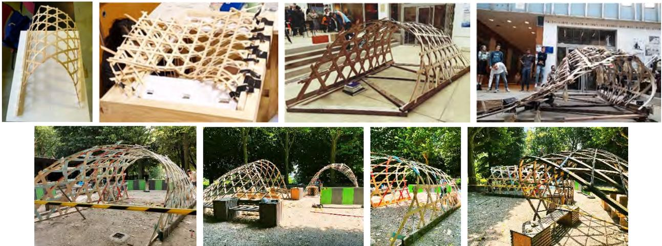
Fig. 26 Load tests on the 1:10 and 1:2 physical models of the Kagome gridshell (single and double layer), and view of the scale 1 pavilion during construction.
