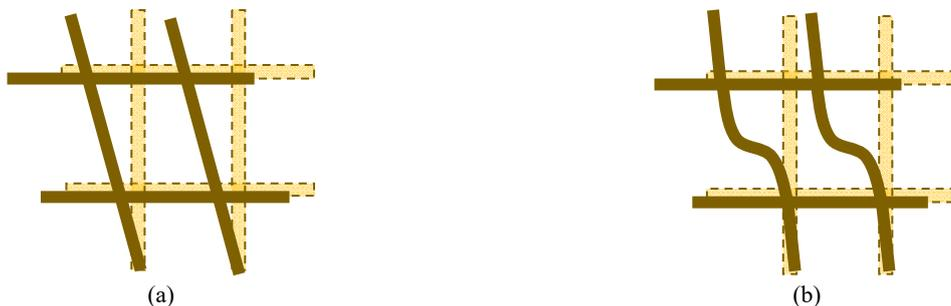
Fig. 17 (a) Hinged nodes; (b) semi-rigid nodes: bending in the plane of the lattices is only possible if the nodes are semi-rigid.
