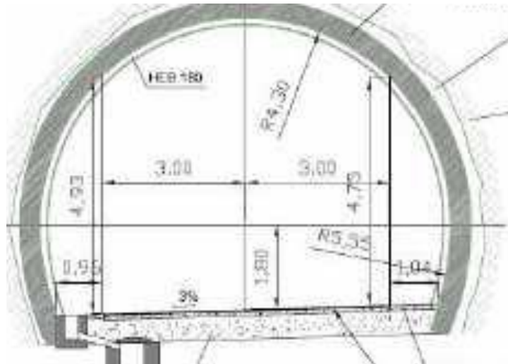
Fig. 1 Section of the “Tunnel du Roux”.
