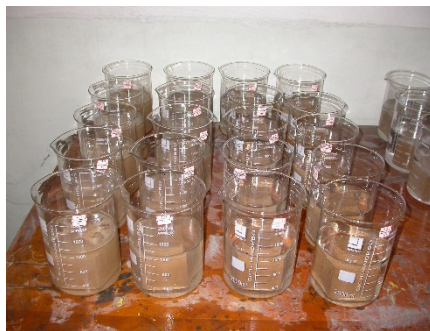
Fig. 1 Cemented soil samples and MgSO_4 solutions.
