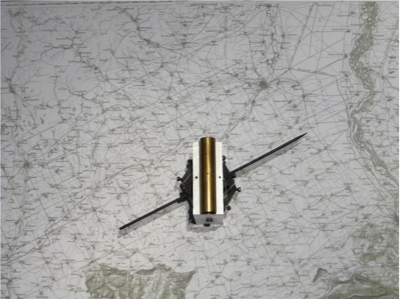
Fig. 7 Positioning the axle of the starfinder-tube parallel to the axis of rotation of the dodecahedron will result in ENE-alignments of 63,435^\circ from N.
