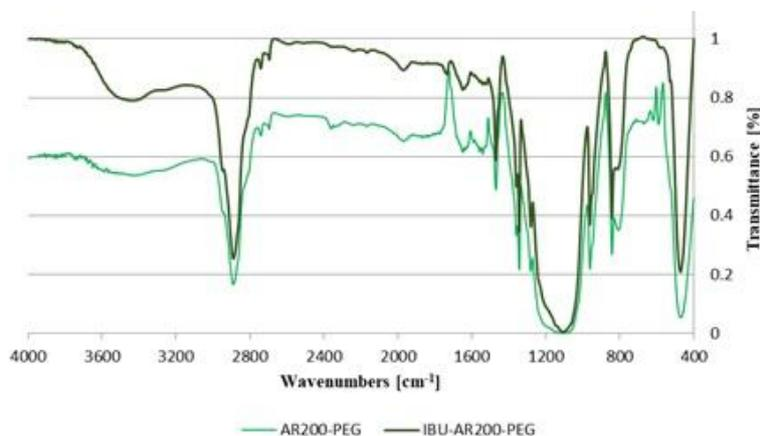
Fig. 6 FTIR spectra for Aerosil 200A compositions (KBr disk).
