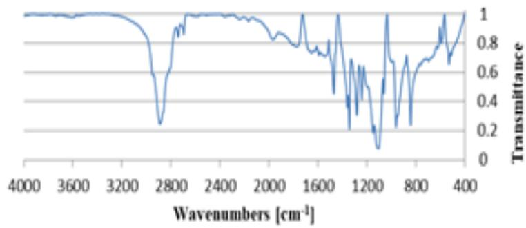
Fig. 2 FTIR spectrum for polyethylene glycol (KBr disk).
