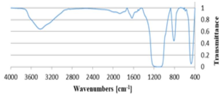
Fig. 4 FTIR spectrum for Aerosil 200V (KBr disk).
