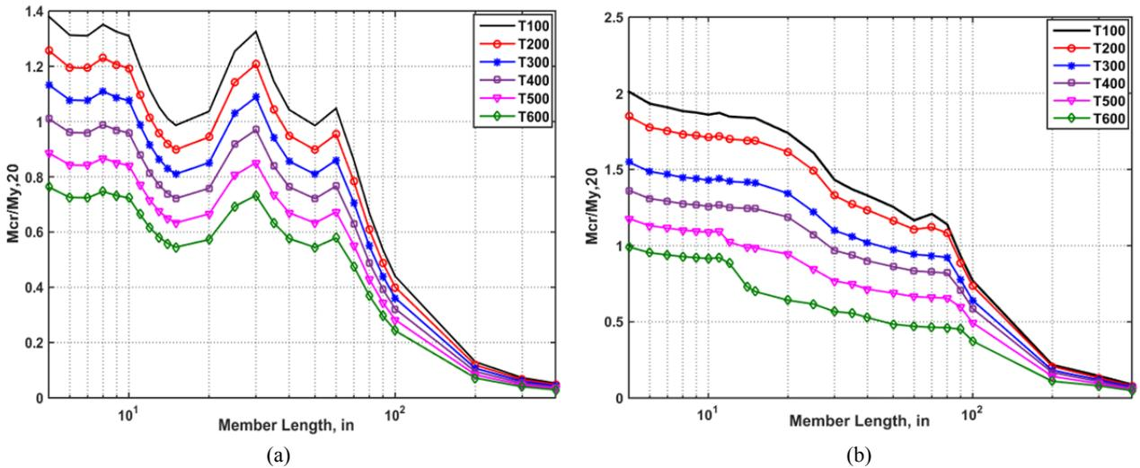
**Fig. 6 Normalized critical buckling moment for section 600S200-54 (a) uniform and (b) non-uniform.**
