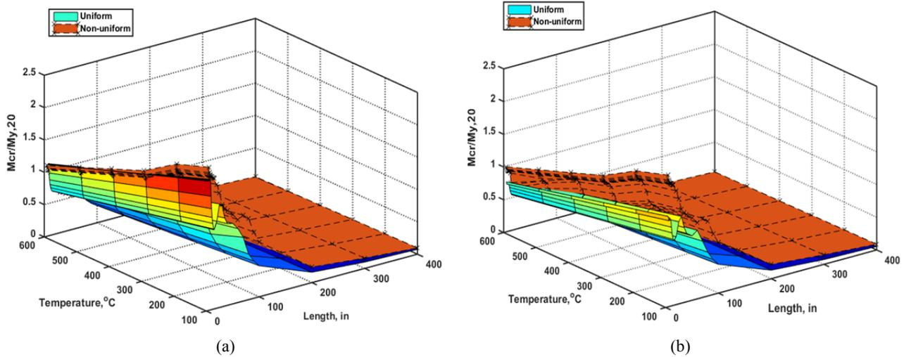
Fig. 7 Critical moment comparison under uniform and non-uniform temperature distribution for section (a) 362S200-54 and (b) 600S200-54.
