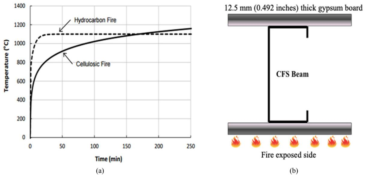
Fig. 1 (a) ISO834 standard fire and (b) CFS channel section protected by gypsum board and fire on one side.
