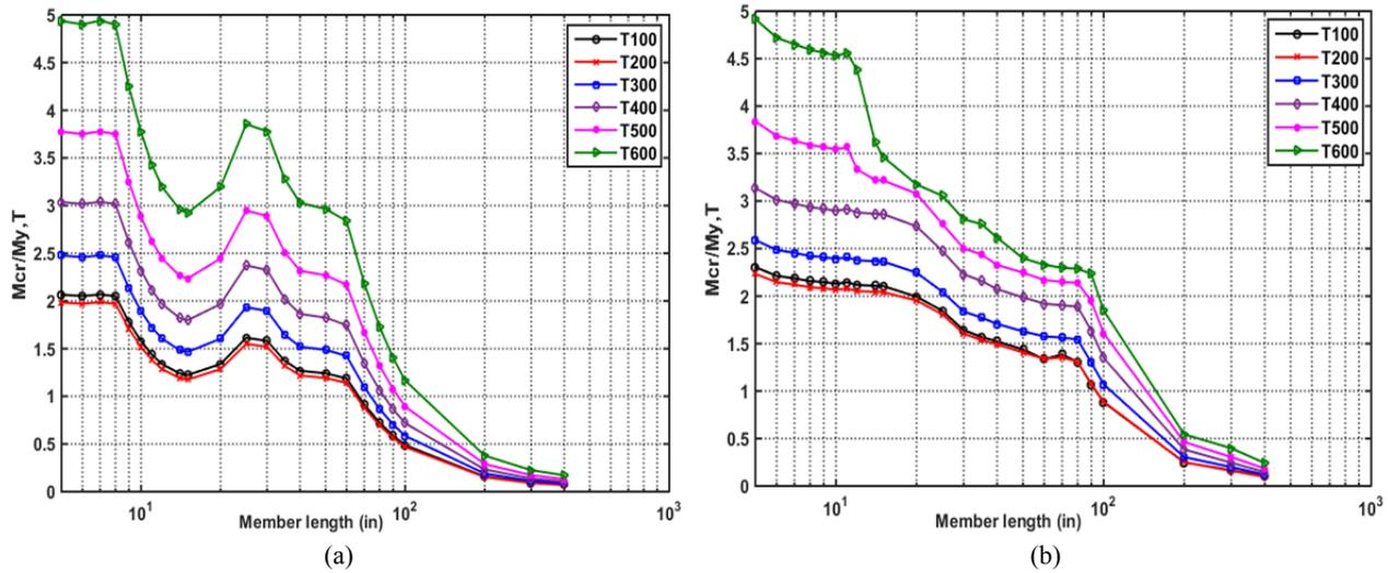
**Fig. 5 Normalized critical buckling moment for section 400S200-54 (a) uniform and (b) non-uniform.**
