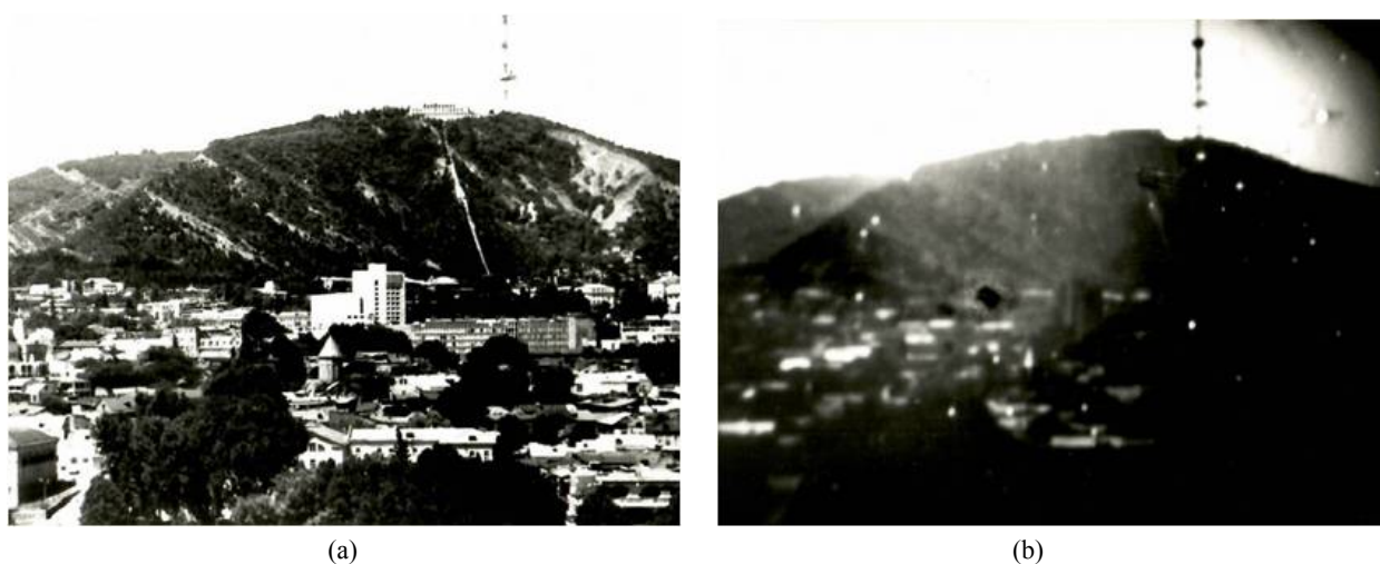
Fig. 13 (a) The usual photo of the city landscape and (b) its polarization image obtained on the material MPY.
