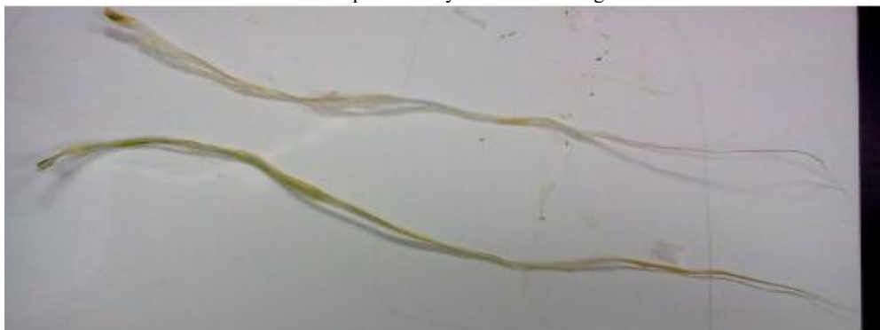
Fig. 2 Samples of microbial retted fibers from Yucca leaves.
