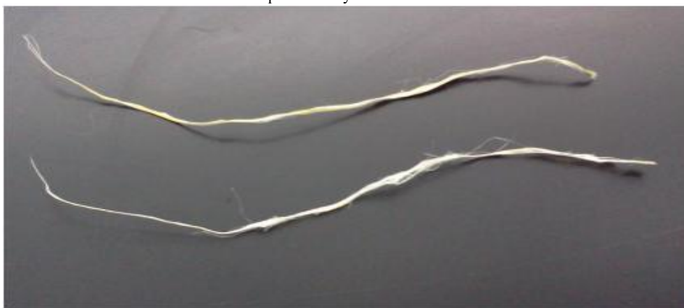
Fig. 1 Samples of chemically retted fibers from Yucca leaves.
