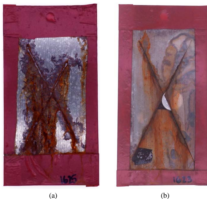
Fig. 1 The coating on steel panels after salt fog test (ASTM b 117, ~200 h): (a) without cation exchange resin, and (b) with cation exchange resin,
