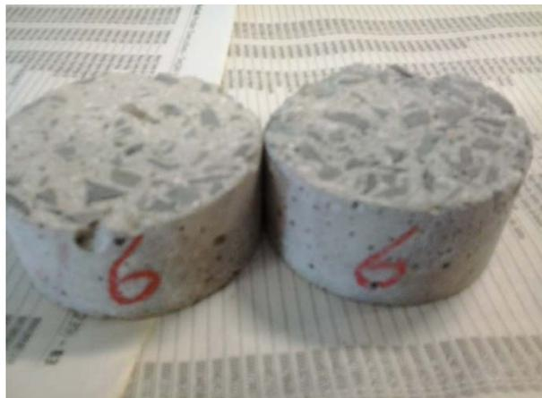
**Fig. 2** Samples 50 mm diameter and 25 mm of height obtained from the cylindrical samples ( $D$  = 50 mm and  $h$  = 25 mm) for the Thermal conductivity analyses.
