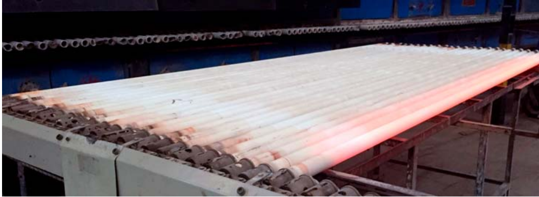
Fig. 4 Roller kiln's cordierite roller materials [5].
