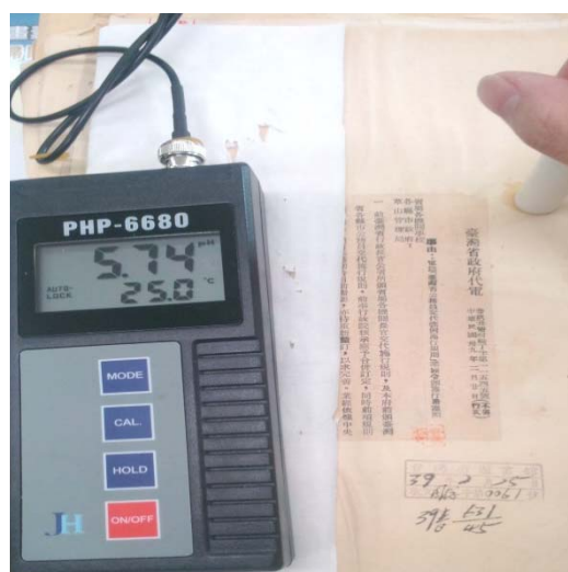
Figure 2. On Apr. 16th 2014, Pineapple Xuan Papers were used to wrap archives with interleaves inserted for one week to test the variation of PH value of archives dated 1950 before and after experiment.
