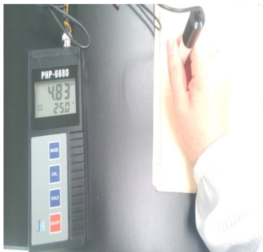
Figure 1. On Apr. 11th 2014, Pineapple Xuan Papers were used to wrap archives with interleaves inserted for one week to test the variation of PH value of archives dated 1950 before and after experiment.
