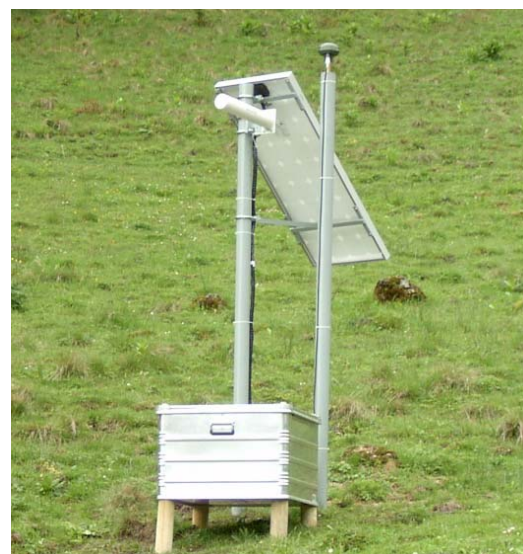
Fig. 2 GNSS sensor node at Aggenalm landslide.
