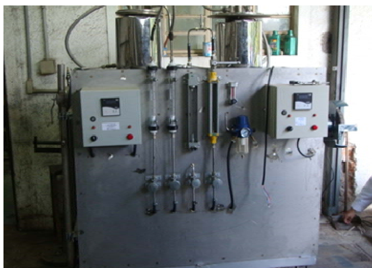
Fig. 3 Picture with the control panel and assembling in tandem of the two molten salt reactors.
