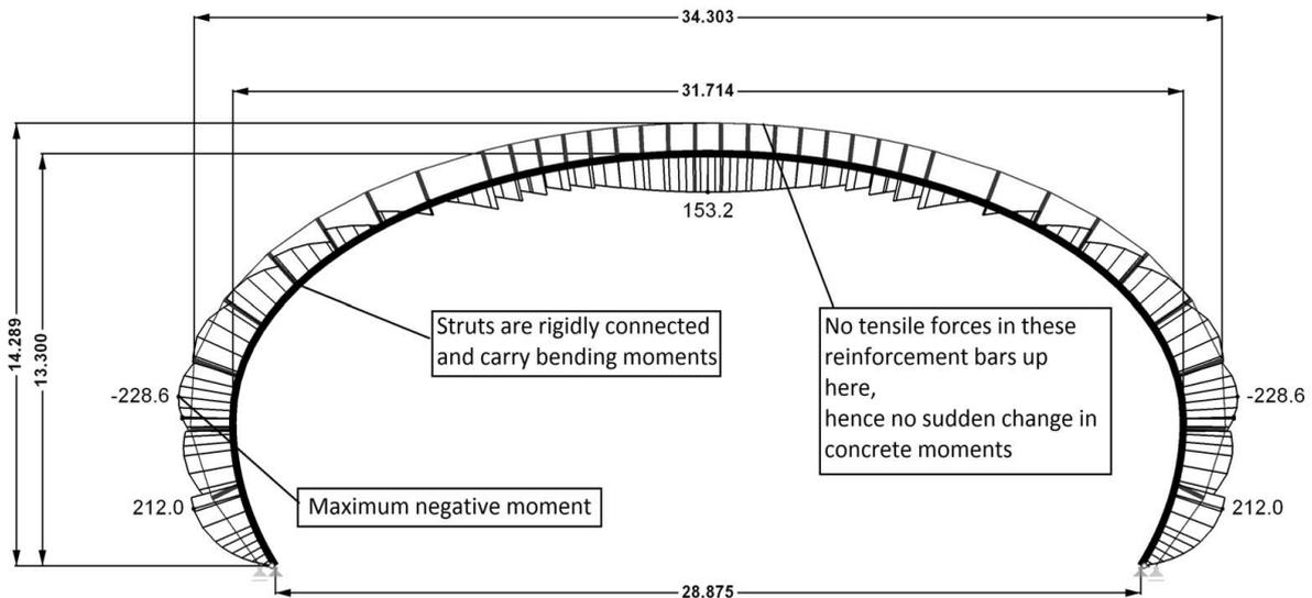
**Fig. 10 Frame on Charles de Gaulle Airport with external tensile reinforcement, bending moment distribution due to self-weight. Struts are rigidly connected to concrete frame and hence tensile and compressive side work more like one single section.**
