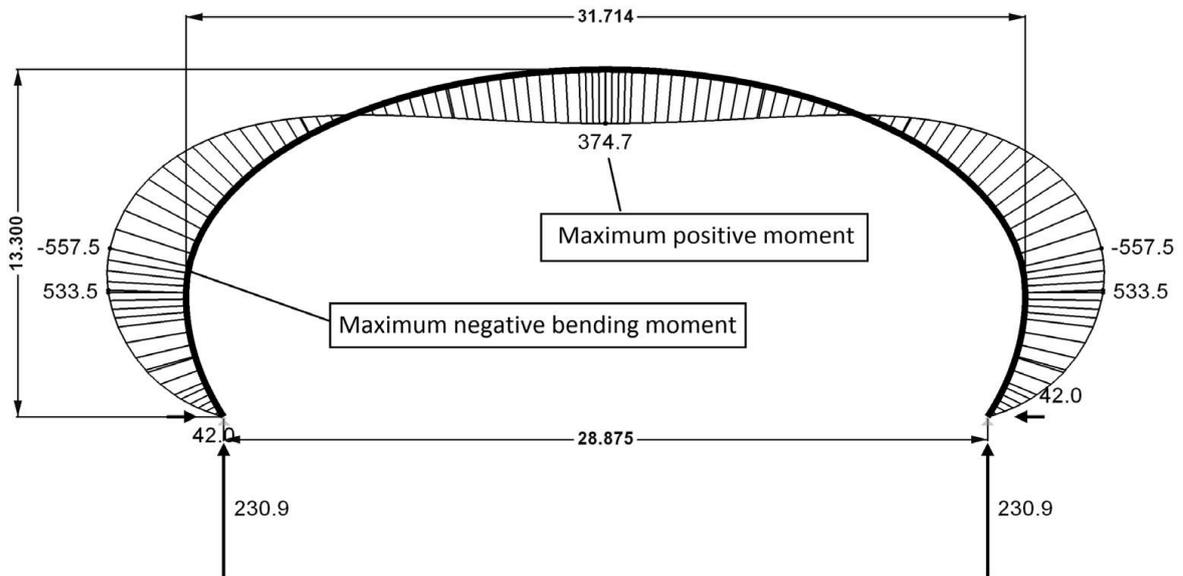
Fig. 7 Base frame geometry based on Charles de Gaulle Airport frame, bending moment distribution and support reactions due to self-weight.
