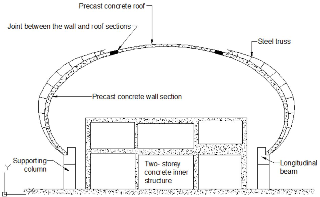
Fig. 5 Cast in place joint between roof and wall elements.
