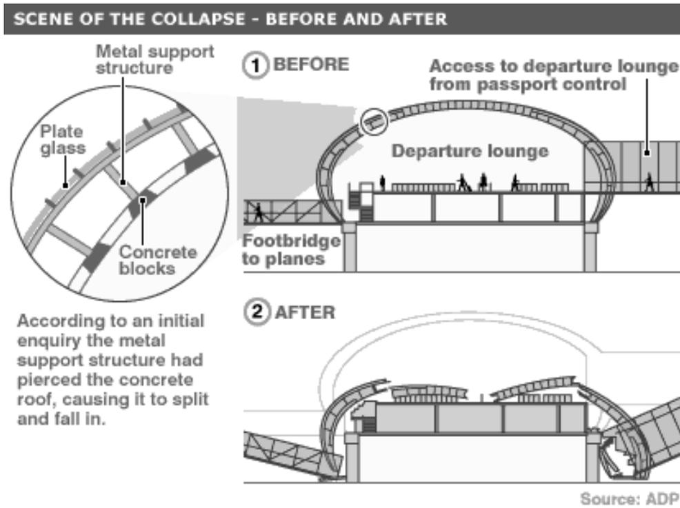
Fig. 1 Charles de Gaulle curved concrete shell reinforced with exterior steel struts.
