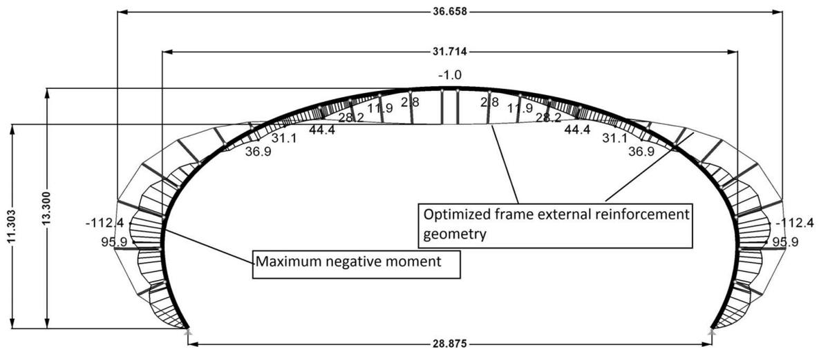
Fig. 9 Frame with optimized external tensile reinforcement, bending moment distribution due to self-weight.
