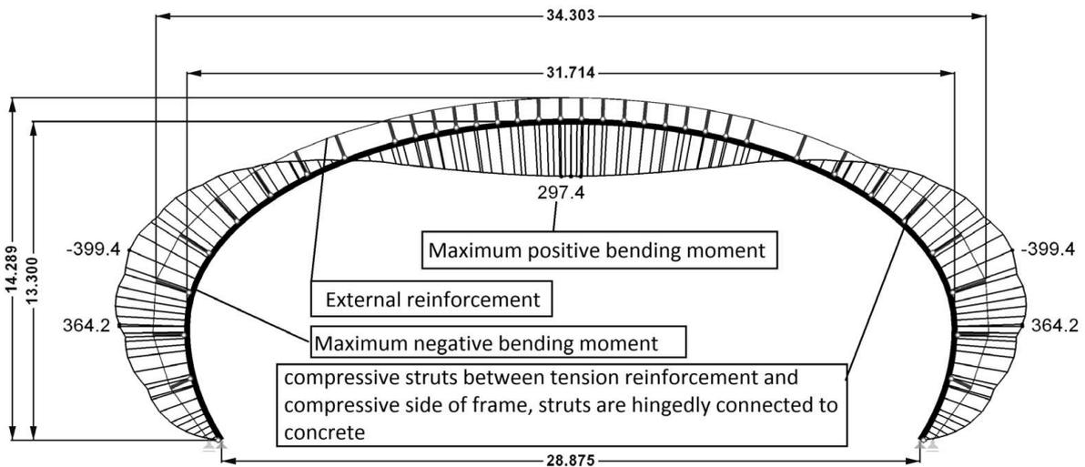
Fig. 8 Frame on Charles de Gaulle Airport with external tensile reinforcement, bending moment distribution due to self-weight.
