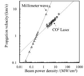
Fig. 5 Propagation velocities of the ionization front at respective beam power densities.
