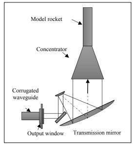
Fig. 4 Long-distance millimeter-wave transfer system with the tapered tube concentrator.
