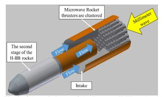
Fig. 8 Schematic image of the Japanese H-IIB replaced the first stage engine and solid rocket boosters by the Microwave Rocket.
