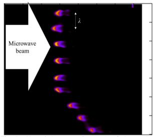
Fig. 7 Numerical computation result of the number density of the electron.
