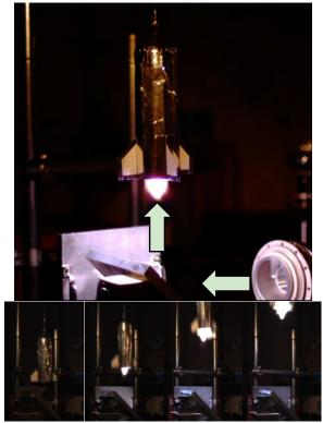
Fig. 2 The 109 g model rocket launch in a multi-pulse operation.
