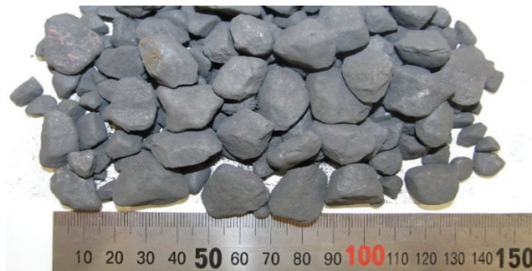
Photo. 1 High-density aggregate ( \mu = 4.5 g/cm 3 ).
