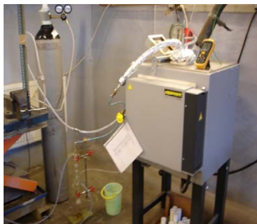
Fig. 1 Experimental set up used for sugarcane bagasse torrefaction.
