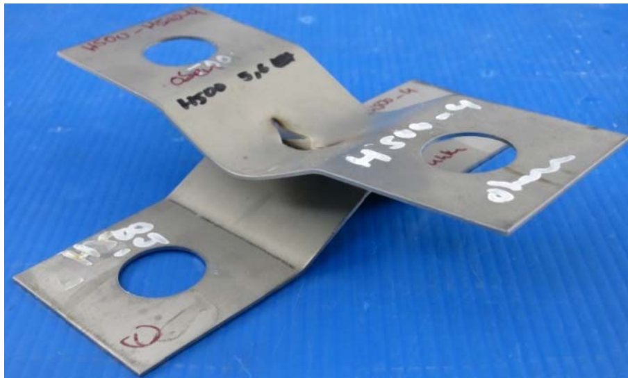
Fig. 4 Ductile behavior of a laser beam welded cross-tensile-sample.
