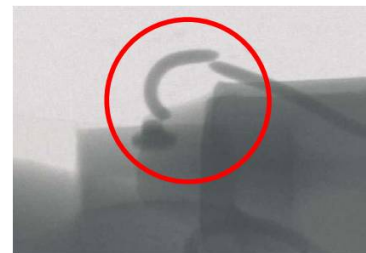
Fig. 14 X-ray inspection point out the wire's break.
