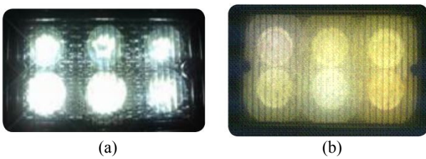
Fig. 11 (a) Silicon resin (new) degrade and turns yellow after (b) VOC exposition (after 100 h), decreasing luminous efficacy.
