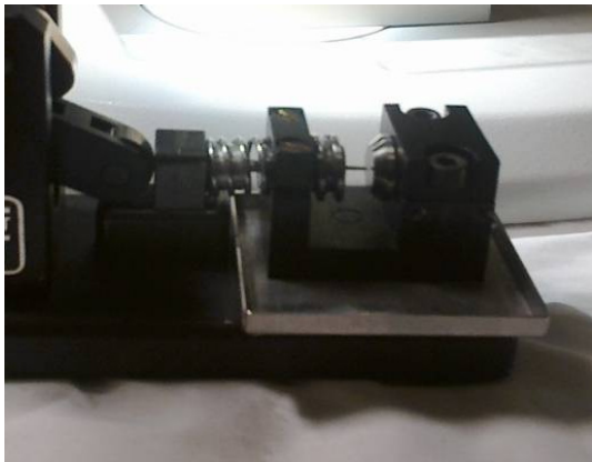
Fig. 7 Novel punching device for 1 mm TEM thin foils.
