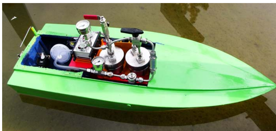
Fig. 4 A model boat as technology demonstrator for electric marine vehicle operation using on-board an Al-water hydrogen reactor and a PEM fuel cell.
