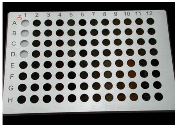
**Fig. 2** Aluminum micro plate used to scan ground soil samples.
