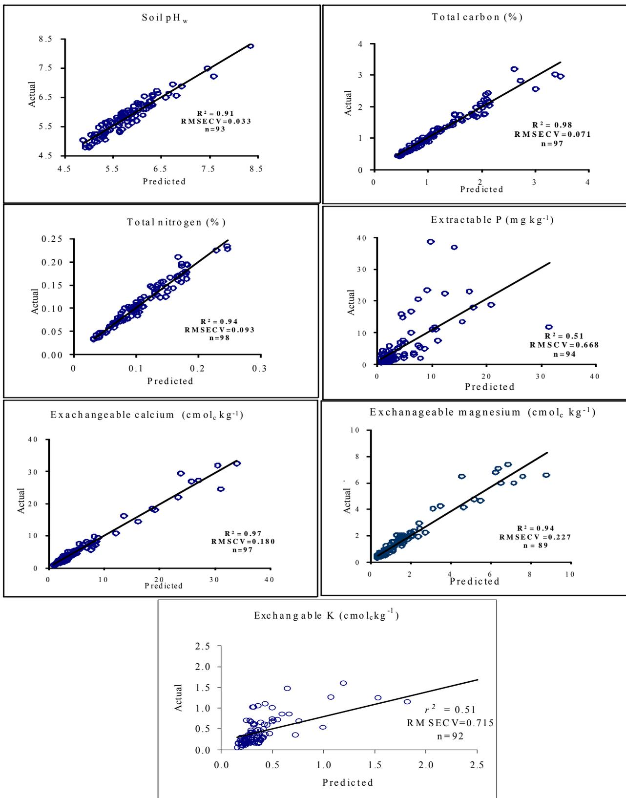
Fig. 3 Cross-validated calibration models for principal soil nutrients: soil pH<sub>w</sub>, total carbon, total nitrogen, extractable phosphorus, and exchangeable calcium, magnesium and potassium.
