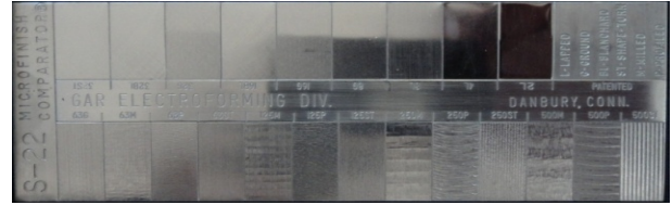
Fig. 1 Microfinish surface roughness comparator.
