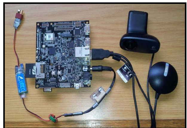
Fig. 2 Assembled monitoring system with sensors.
