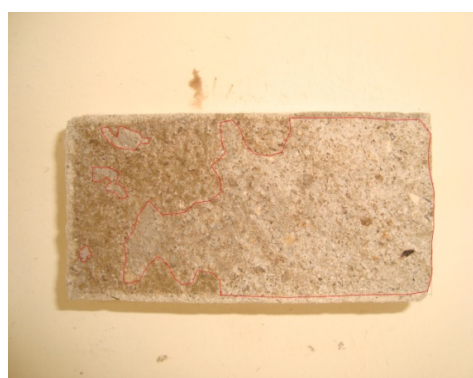
Fig. 5 Part of the whitish surface indicating contamination by free chlorides.
