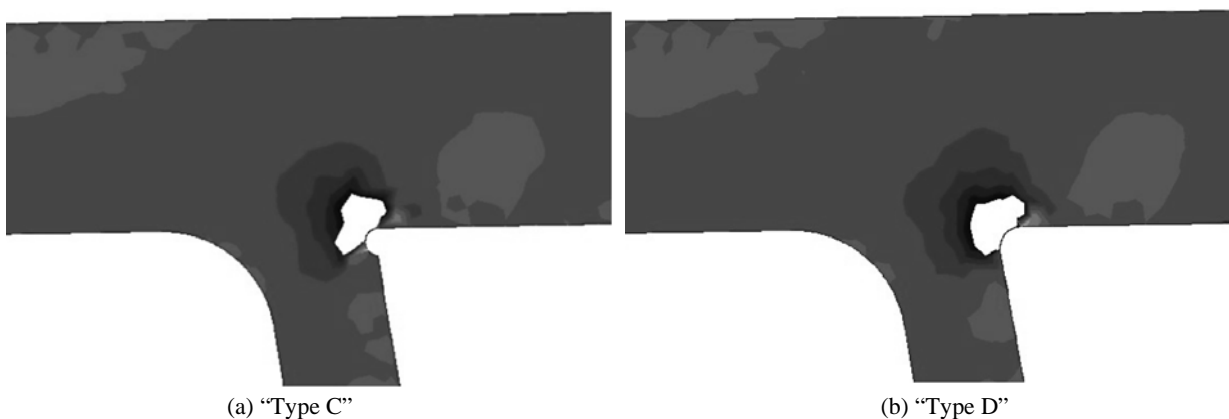
Fig. 10 “Stress peak zone” in the stiffener web to deck plate connection.
