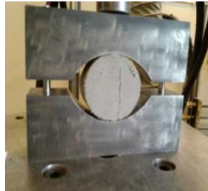
Fig. 13 Brazilian test arrangement with typical tensile fracturing [11].
