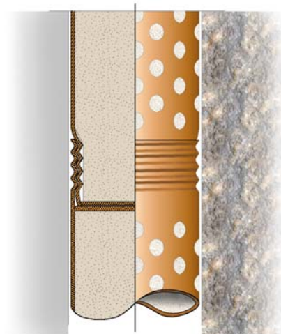
Fig. 3 Perforated copper tube with highly compacted smectite clay, tubes are jointed to form long segments that are inserted in the holes (drawing by Sweco Int. Co.).
