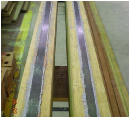
Fig. 3 Strengthened timber beams being cured.
