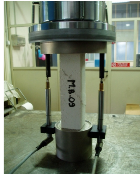
Fig. 5 Compression test on single mortar specimen.
