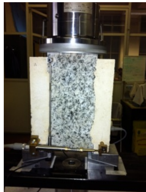
Fig. 10 Composite specimen stone-repair mortar.
