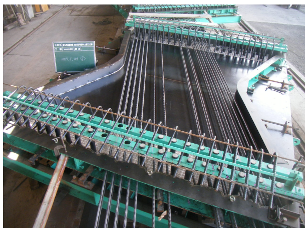
Fig. 8 Fabrication stage of panels.
