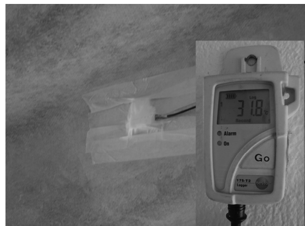
Fig. 6 Surface temperature sensor under the tile (individual sensor and mini logger).
