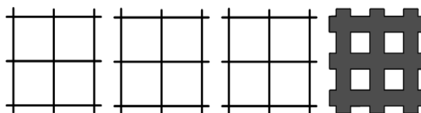
Fig. 4 The ANSYS FEM thermal model geometries of UO 2 -BeO nuclear fuels with 0.6, 0.9, 1.2 and 13.6 wt% of BeO as generated by an automated program.
