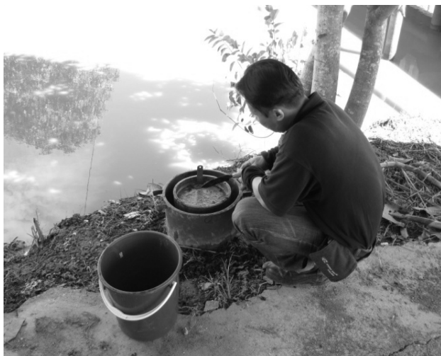
Fig. 4 Field infiltration test using double ring infiltrometer.
